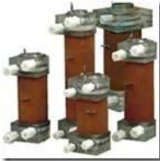
Round water electrolyzer cells provide the greatest area of electrode surface with the highest possible electrolysis efficiency. The anode and cathode consist of two tubular cylinders of titanium, one inside the other. A ceramic membrane separates the two. The membrane prevents mixing of the two electrolyzed water solutions that are co-produced.
