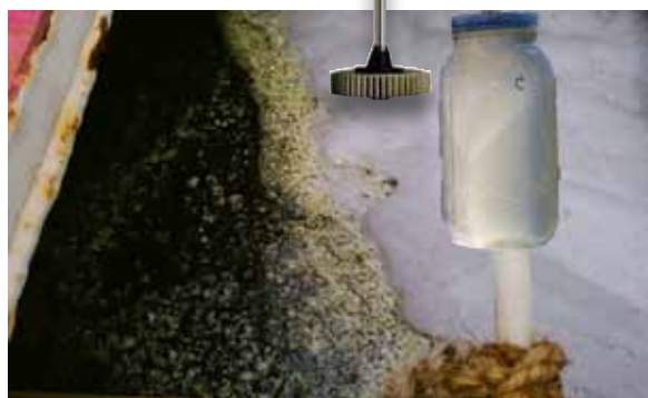
Above: The turbine aerator can be considered a means of pretreatment for black water remediation. Below: This split image shows the frac cure tank before and after turbine aeration.
